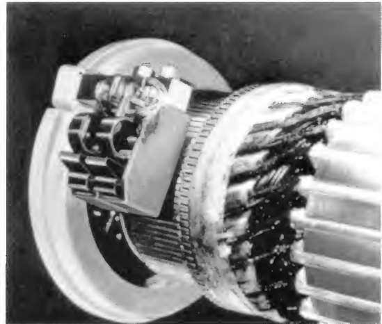
Figure 4.35 a. Carbon brush and ultraflexible copper lead. b. Brush holder and spring to exert pressure. c. Brush set composed of two brushes, mounted on rocker arm. (Courtesy of General Electric Company, USA)
