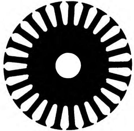
Figure 4.31 Armature lamination with tapered slots.
