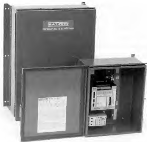
Figure 23.23b Solid-state soft starter rated 5 hp, 460 V, 60 Hz. Start-up time adjustable 5–50 s; initial torque adjustment 0–75%; current limit schedule 75%–400%; kick-start time adjustable 0–1.5 s. In background is 40 hp, 460 V soft starter. (Courtesy of Baldor Electric Company)
