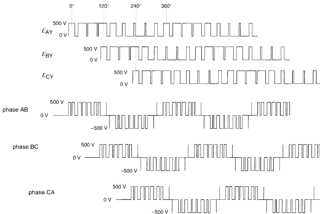
Figure 21.88 Three-phase PWM voltages produced by a dc-to-ac switching converter operating at 540 Hz with a 500 V dc input. Top: E_{AN} , E_{BN} , E_{CN} outputs, peak 60 Hz sinusoidal component = 200 V. Bottom: E_{AB} , E_{BC} , E_{CA} outputs, peak 60 Hz sinusoidal component = 346.4 V, rms value = 245 V.
