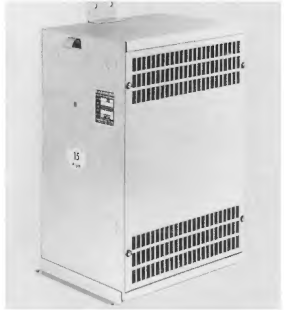
Figure 10.15 Single-phase dry-type transformer, type AA, rated at 15 kVA, 600 V/240 V, 60 Hz, insulation class 150°C for indoor use. Height: 600 mm; width: 434 mm; depth: 230 mm; weight: 79.5 kg. (Courtesy of Hammond)
