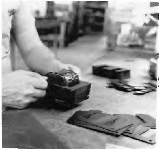
Figure 10.9b Stacking laminations inside a coil.
