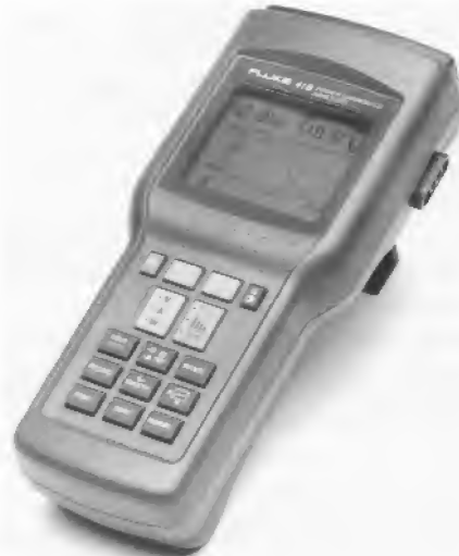
Figure 30.45 This portable instrument, the “Power Harmonics Analyzer” can measure the total harmonic distortion (THD) of a voltage or current up to the 31 st harmonic. It can also measure the active, reactive and apparent power in a 3-phase circuit, and its power factor. It also gives a readout of the K factor of a current ( courtesy of Fluke Electronics Canada Inc. ).
